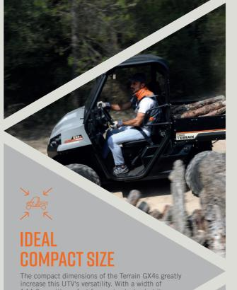
The compact dimensions of the Terrain GX4s greatly increase this UTV's versatility. With a width of 144.9 cm, it's perfect for service tasks, but it can also be used in woodland areas. A perfect size that goes hand in hand with a maximum total load capacity of 440 kg - a leader in its class.
